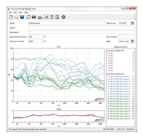
• Verify the measurement data and delete any false readings from the **Measurements** list on the right.
