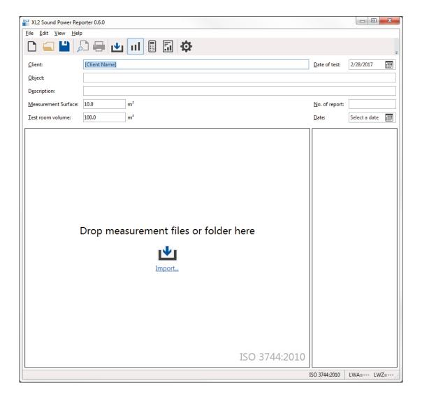
Kindly ensure, prior the data import, that the device folder contains all required measurement data (\*.txt) and \*.xl2 system files of each recorded measurement.
